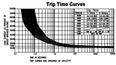
100% of rated current: Hold, No-Trip 135% of rated current : Trip in 1 Hour 200% of rated current: Within 40 Seconds 300% of rated current: Within 10 Seconds
